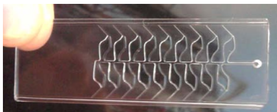
Figure 1. Developed \mu TAS chip for the method. After coating, the chip was covered with a transparent foil-tape.
